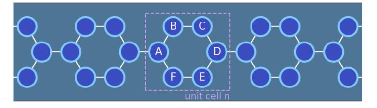
The amplitude of the field in each waveguide can be described by a discrete nonlinear Schrödinger equation:
